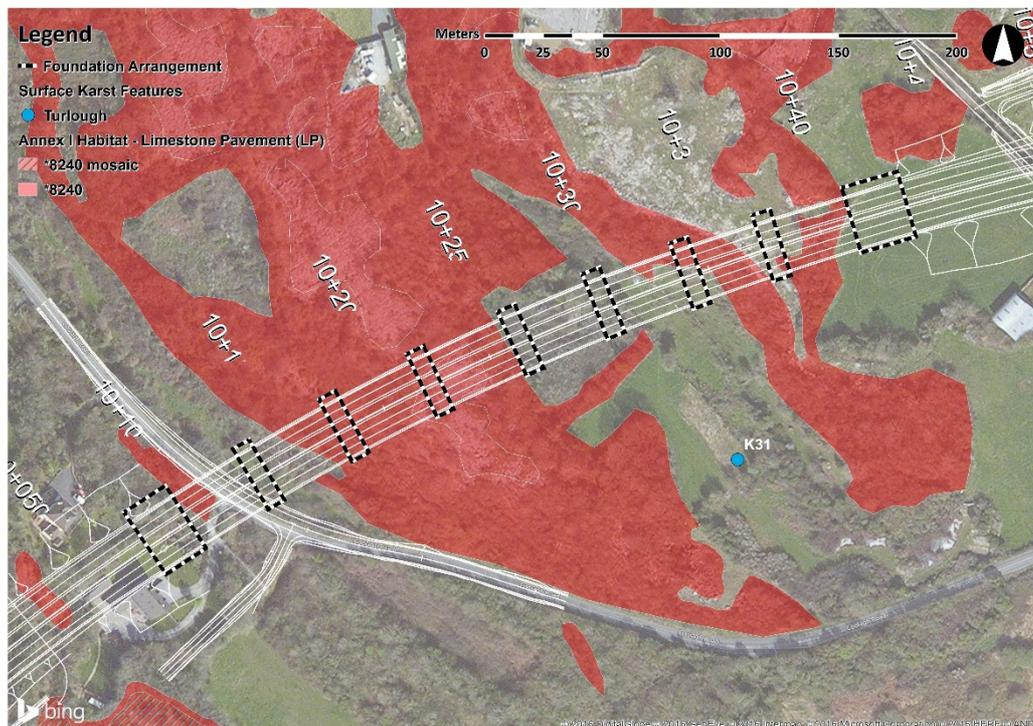
On the western extent of the Annex I habitat, from Ch. 10+150 to 10+200, a zone of low resistivity is observed in the geophysical survey. The drop in resistivity suggests the possibility of karst activity in the underlying limestone.
